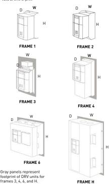
Frame 1-4 have integral cooling fan assemblies where required. Optional ducting kit for cubicle roof external ventilation available for frame 4. Frame Size H has fan cooling assembly that can be cubicle roof mounted or drive mounted. Add 5.9" (150mm) to overall height for drive mounted option.
